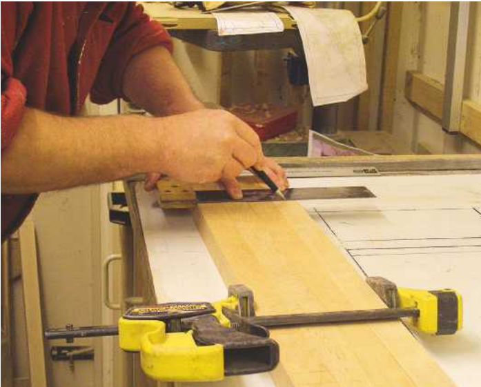
▲ Pic.4 Having planed the legs to size, clamp them together and mark the positions for the joints
